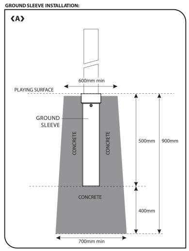
**NOTE:** Recommended foundation sizing only. Actual foundation depends on local ground conditions.
